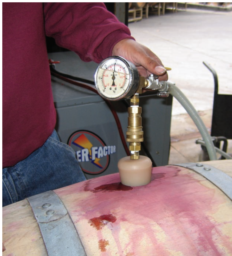
Figure 4. Air being evacuated from the barrel to enhance the extraction of viable Brettanomyces cells from the surface and pores of the staves by sterilised alcoholic (12% v/v) saline solution.
