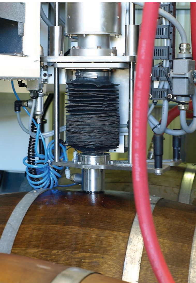
Figure 1. A barrel being sonicated using Cavitus' HPU barrel cleaning and disinfection system. Ultrasound is delivered by a sonotrode inserted through the bung-hole into a barrel filled with water at 60°C. Tartrate removal and destruction of spoilage micro-organisms occurs simultaneously. Water after cleaning is filtered and reused up to 100 times.
