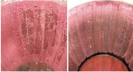
Figure 4. The surface of a five-year-old barrel before cleaning by Cavitus' high power ultrasonic (HPU) technology system on the left (the tartrate deposit is thick, hard and crusty). The photo on the right shows the uniformly cleaned surface of the barrel after eight minutes sonication time by HPU.
