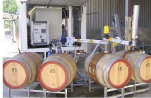
Figure 2. Cavitus' HPU mobile barrel cleaning and disinfection system (patent pending). Simultaneously, the barrel on the right is being sonicated, while the one next to it is being emptied, and an uncleaned barrel (second from left) is being filled. Ultrasound is delivered via a sonotrode inserted through the bung hole into the barrel that is filled with water at 60°C. Tartrate removal and destruction of Brettanomyces occur simultaneously during sonication. Water that is used for cleaning can be reused up to 100 times.
